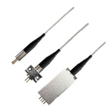
The FPLD series fiber-coupled laser diodes are designed with a GaAs quantum well structure. These diodes feature a built-in photodiode for precise monitoring and feedback control of the laser's output power. Housed in standard TO packages, these diodes are pigtailed to a 1-meter long single-mode fiber terminated with an FC/APC connector. Each unit undergoes rigorous testing prior to shipment to ensure reliability.
